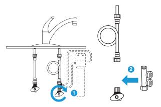
8 Connect 3/8" tubing to the bottom port. Measure tubing to system inlet (marked "IN") and cut to length. Repeat this step for the top port and outlet (marked "OUT").
