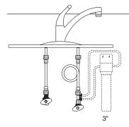
2 Locate a suitable area under the sink to mount the system, noting that at least three (3) inches of clearance from the base of the cartridge is needed for easy cartridge replacement. The System Head must be installed less than three (3) feet from the cold-water inlet valve.
