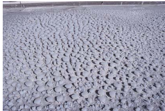
As the zeolite cures, the beds start to shrink and crack and the crystals begin to form.
